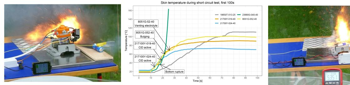
Hard short-circuit tests and overcharging tests:
