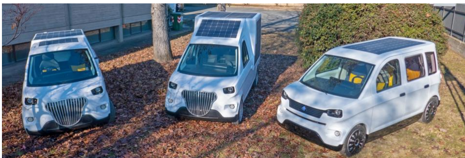
Fig. 1. The Multi-Moby vehicles, currently under development; from the left: Multi-Moby pick-up, Multi-Moby van for food delivery, and Multi-Moby passenger vehicle.
