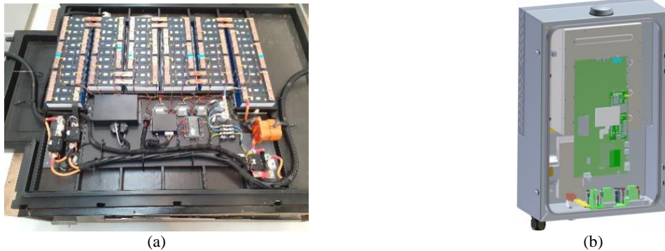
Fig. 9. (a) LFP prismatic cells in a 100 V configuration; (b) 7 kW DC wall box charger, with front door removed.
