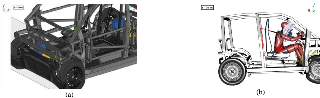
Fig. 2. (a) Simulation results of the Multi-Moby vehicle under R137 crash after structure optimisation; (b) analysis of restraint system under R137.
