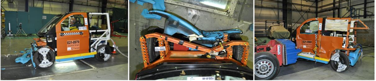
Fig. 3. Crash test aftermaths of three Multi-Moby prototype vehicles, from left to right: R137, R94 and R95.
