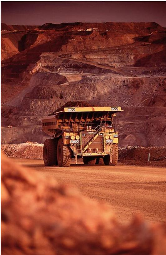
On the road towards decarbonization in the mining industry, going electric is one of the main options to reach zero-emission mining. Currently a mining truck consumes 135 liter diesel per hour. We replace it with a battery that can deliver 2 MW in power and can be used with a variety of fast charging options.
