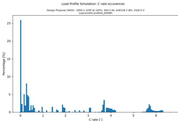
The C-rate is on average 2C with peaks up to 6.9C while charging and 4.4C while discharging. In general, the battery load is relatively low. This will increase as the battery ages but remains well within the maximum values.
