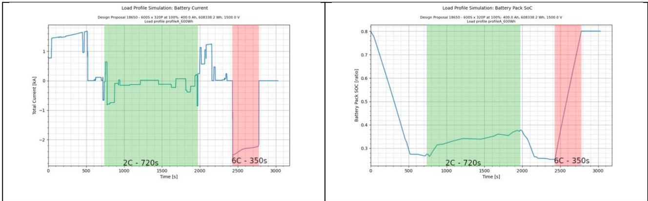
The graphs above show the evolution of the current and the evolution of the SoC level of the battery for the selected set-up. If for example it would be feasible to charge with higher currents on the overhead charging segment, then the end-of-trip charging time can be further reduced.
