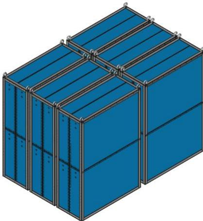
The battery is constructed from 24 modules, divided over 4 lifting frames, resulting in compactness and modularity. Each frame contains four 25kWh modules. They will fit in a 2.6m x 1.8m x 1.9m space. The proposed solution requires 9 m<sup>3</sup> with a total mass of 13 ton.
