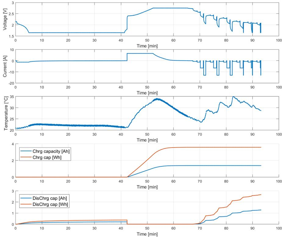
What are the conclusions? The cell charges at a constant current of 5C in about 10 minutes to reach 75%. The test sequence can be fully repeated 3 times and partly a 4<sup>th</sup> and 5<sup>th</sup> and 6<sup>th</sup> time with the temperature never reaching more than 35°C. Hence, no need for cooling. The first three runs take about 75% of the cell's capacity.
