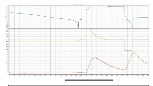
Test 4728 - 18650 cell - charge at 10C (13A) - discharge at 10C (13A) room at 25°C +/- 2 °C Maximum temperature increase: +22 °C Energy injected: 3,59 Wh in 850 seconds Energy released upon discharge: 2,28 Wh in 315 seconds DOD: 88%
