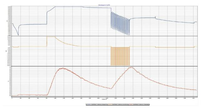
Test 4744 - 18650 cell - charge at 10C (13A) - discharge pulsed at at 20C (26A) - room at 25°C +/- 2 °C. Average discharge current 6,24 A (4,8C) Pulse: discharge for 6 seconds at 20C (26A) then for 24 seconds at 1C (1.3A) and repeat until voltage drops to minimum. Maximum temperature increase: +12.5 °C
