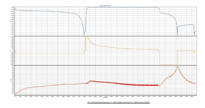
Test 4737 - 18500 cell - charge at 5C (5A) - discharge at 5C (5A) room at 45°C +/- 2 °C Maximum temperature increase: +9.5°C Energy injected: 3,09 Wh in 2626 seconds Energy released upon discharge: 2,734 Wh in 656 seconds DOD: 91%
