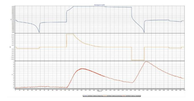
Test 4734 - 18650 cell - charge at 10C (13A) - discharge at 10C (13A) room at 25°C +/- 2 °C Maximum temperature increase: +15 °C (use of heat absorbing material)
