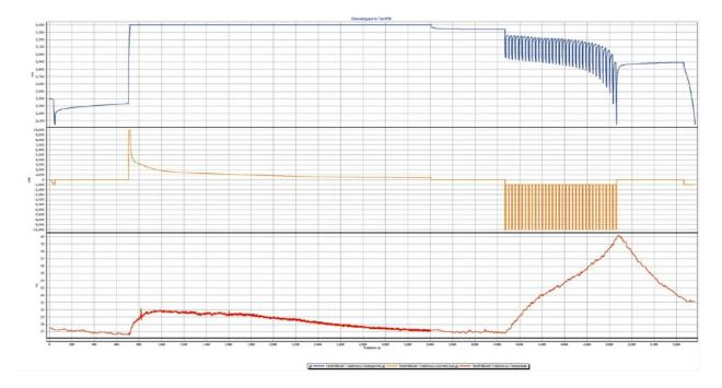
Test 4745 - 18500 cell - charge at 10C (10A) - discharge pulsed at 10C (10A) room at 25°C +/- 2 °C. Average discharge current 2,6A (2,6C).
