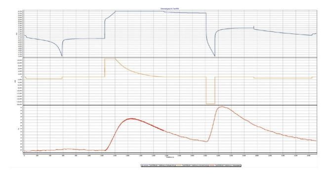
Test 4740 - 18650 cell - charge at 10C (13A) - discharge at 20C (26A) room at 25°C +/- 2 °C Maximum temperature increase: +13.5 °C (use of heat absorbing material) Energy injected: 3,61 Wh in 909 seconds Energy released upon discharge: 1,36 Wh in 135 seconds. DOD: 75%
