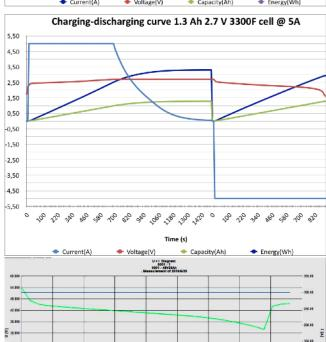
The 18650 power capacitor cell can contain about 3.2 Wh at 2.7 V. (100 Wh/kg). Charged in about 12 minutes to 80% capacity or to 100% in 25 minutes at 5A. However, this power capacitor can also be charged and discharged at 10 A without any significant heat generation. Higher short bursts of up to 100 A are permitted.
