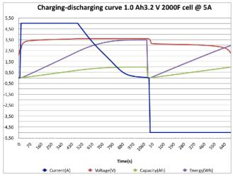
The 18500 power capacitor cell can contain about 3.4 Wh at 3.2 V. (80 Wh/kg). Charged in about 10 minutes to 80% capacity or to 100% in 20 minutes at 5 A. However, this power capacitor can also be charged and discharged at 20 A without any significant heat generation. Higher short bursts of up to 100 A are permitted. It has an estimated lifetime of 20000 cycles.
