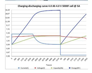
This 23680 power capacitor cell can contain about 16 Wh at 4.0 V. (200 Wh/kg). Charged in about 60 minutes to 80% capacity or to 100% in 120 minutes at 5A. Higher short bursts of up to 8 A are permitted.
